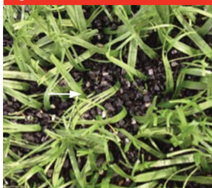
Photograph of a third-generation artificial playing surface. Note the long artificial blade length and the black crumbled rubber base (arrow).
